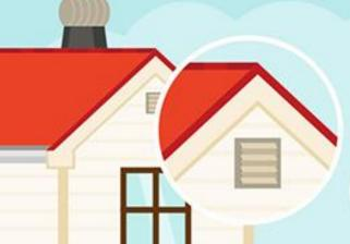
A critical factor to roof durability is proper ventilation. Attic airflow prevents structural damage caused by moisture, reduces energy consumption and increases roof lifespan.
